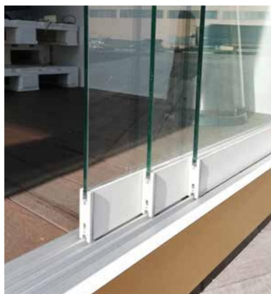
The new MyGlass system of full sliding glass doors can be used on Pergotenda® and bioclimatic pergola ranges. MyGlass uses 10 mm tempered glass and extruded aluminium runners, and can reach a maximum size of 10 x 3 m in its version with 4 ways and 8 doors. The painted aluminium door profile is equipped with caps that facilitate the movement of the windows during opening and closing.
